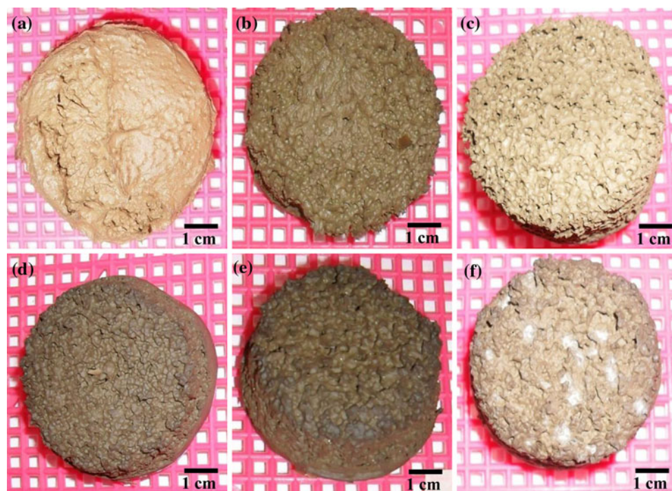
Fig. 4 Porous green bodies consolidated with different forming conditions. Upper panel 11 wt% corn starch-loaded ceramic slurries with yeast additions of a 8.9 wt%, b 17.4 wt%, c 31.5 wt%. Lower
